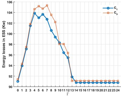
Fig. 14. The round trip losses of ESS vs  $\Gamma$  in case C: Active power losses payments minimization (using ESS  $C_1$ , using both DR & ESS  $C_3$ ).
