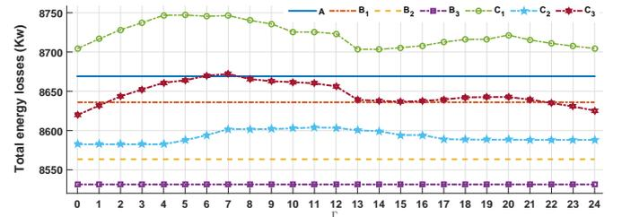
Fig. 13. The active energy losses vs  $\Gamma$  in different cases. A: no ESS/DR, B: loss minimization (using ESS  $B_1$ , using DR  $B_2$ , using both DR & ESS  $B_3$ ), C: loss payments minimization (using ESS  $C_1$ , using DR  $C_2$ , using both DR & ESS  $C_3$ ).
