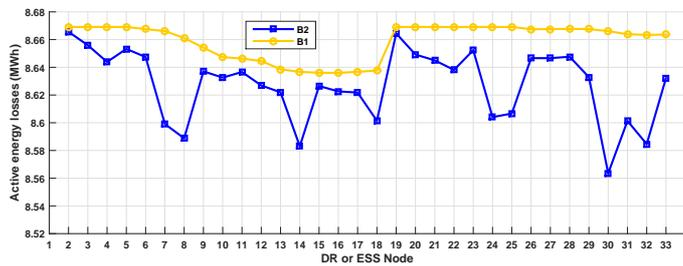
Fig. 5. a) The impact of ESS connection node on active losses (case  $B_1$ , loss minimization using ESS). b) The impact of DR connection node on active losses (case  $B_2$ , loss minimization using DR)
