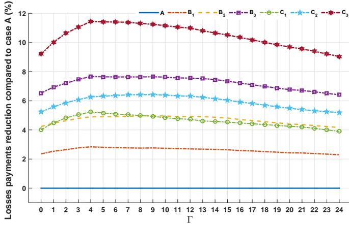
Fig. 4. The energy losses payment reductions (%) vs  $\Gamma$  in different cases. A: base case, B: loss minimization (using ESS  $B_1$ , using DR  $B_2$ , using both DR & ESS  $B_3$ ), C: loss payments minimization (using ESS  $C_1$ , using DR  $C_2$ , using both DR & ESS  $C_3$ ).
